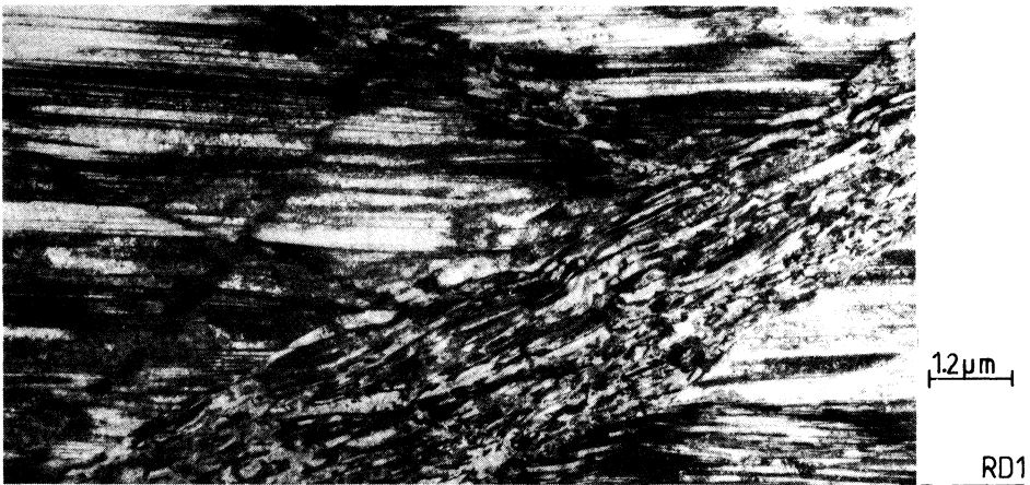
Figure 3 TEM micrograph of the 80% cross rolled specimen (longitudinal section)
