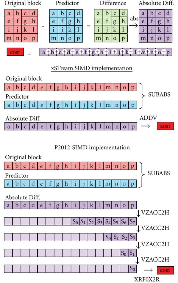
FIGURE 9: Predictor cost calculation.
