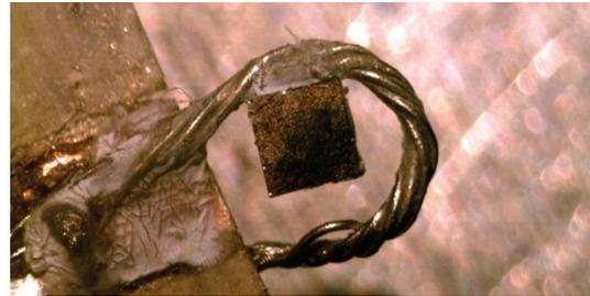
FIGURE 9: Field generating coil for characterizing the Faraday rotation of preferential domains.
