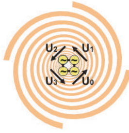
FIGURE 30.9. Geometry of a spiral antenna with voltage sources between the single arms of the spiral.
