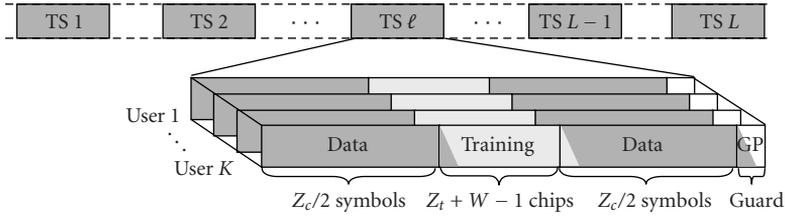
FIGURE 3.6. Block-by-block transmission in hybrid TD-CDMA systems.
