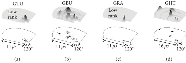
FIGURE 3.7. Power-delay-angle profile for channels generated according to COST-259 DCM propagation environments: (a) GTU, (b) GBU, (c) GRA, and (d) GHT.
