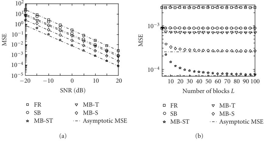
FIGURE 3.4. MSE of the SB and MB subspace-based estimates in spatially correlated noise (a) for varying SNR and  $L = 40$  and (b) for varying  $L$  and SNR = 20 dB.
