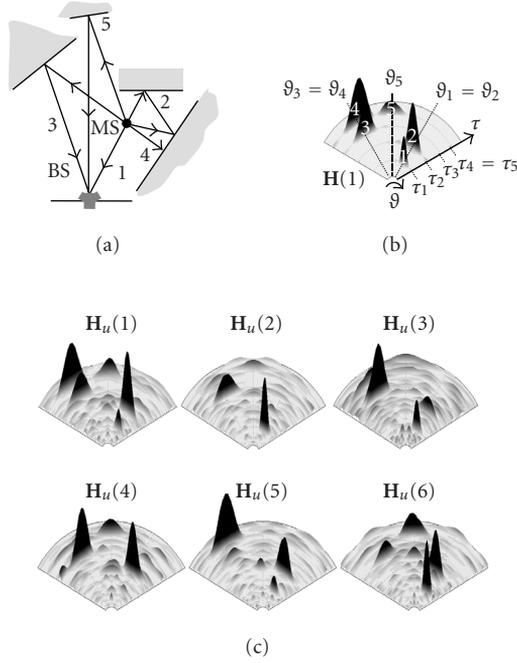
FIGURE 3.2. Example of block-by-block unconstrained estimation for a block-faded channel with stationary angle-delay pattern: (a) multipath model with  $P = 5$  paths,  $q_S = q = 3$  and  $q_T = 4$ ; (b) power-delay-angle diagram for the channel in the first block; and (c) power-delay-angle diagram for the unconstrained estimate in six different blocks.
