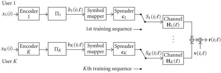
FIGURE 3.10. Transmitter structure for a coded CDMA system.
