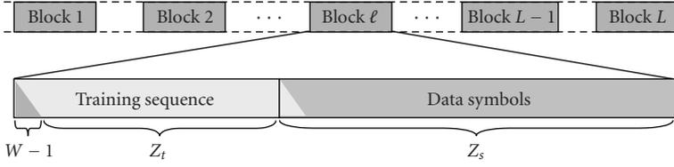
FIGURE 3.1. Block-by-block transmission system.
