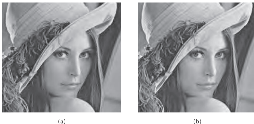
FIGURE 1.9. Reconstruction of “Lena” from 1 : 50 compression files of wavelet coefficients of B9/7 (a) and DS3 (b) transforms.
