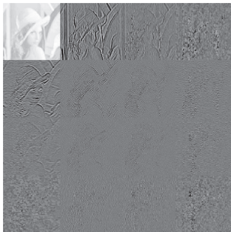
FIGURE 5.21. Subbands of Lena image for sliding window DCT domain image representation in 7 \times 7 pixel-window. Only 16 bandpass filtered images that correspond to 16 ( 4 \times 4 ) basis functions involved in the processing (functions with even indices) are shown arranged in lexicographic order from left to right and from top to bottom.
