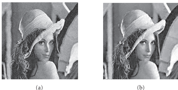
FIGURE 8.26. An example of image denoising and resampling from irregular to regular sampling grid: (a) noisy image sampled in an irregular sampling grid; (b) denoised and resampled (rectified) image.
