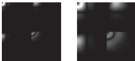
FIGURE 5.24. Last 3 \times 4 2D subbands, shown in spatial frequency coordinates, of the hybrid WL/SWDCT filtering using binom5 wavelets and SWDCT in 3 \times 3 window.
