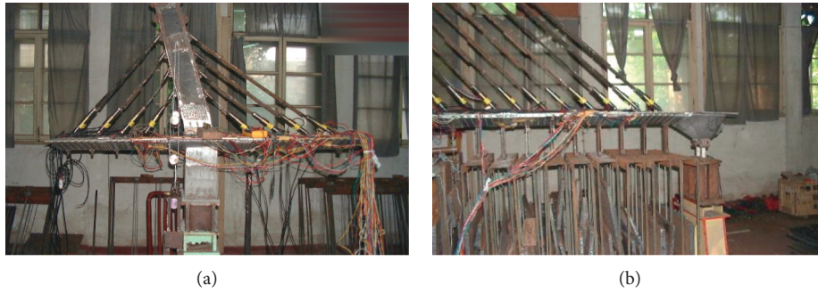
FIGURE 3: Installing the model. (a) Installing four pairs of stay cables at pier #4. (b) Closure of side span of pier #5.
