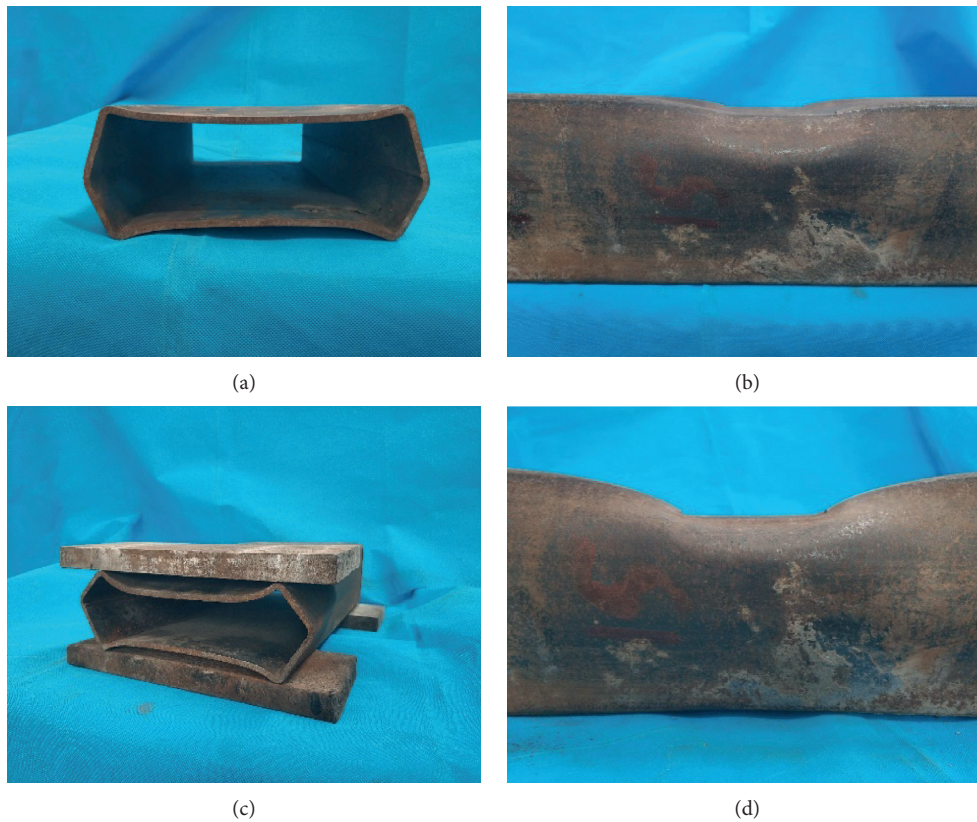
FIGURE 5: Photos of failure modes under four boundary and loading conditions. (a) EOF. (b) IOF. (c) ETF. (d) ITF.
