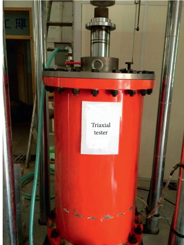
FIGURE 5: ST-1500-type electrohydraulic servo static triaxial tester.
