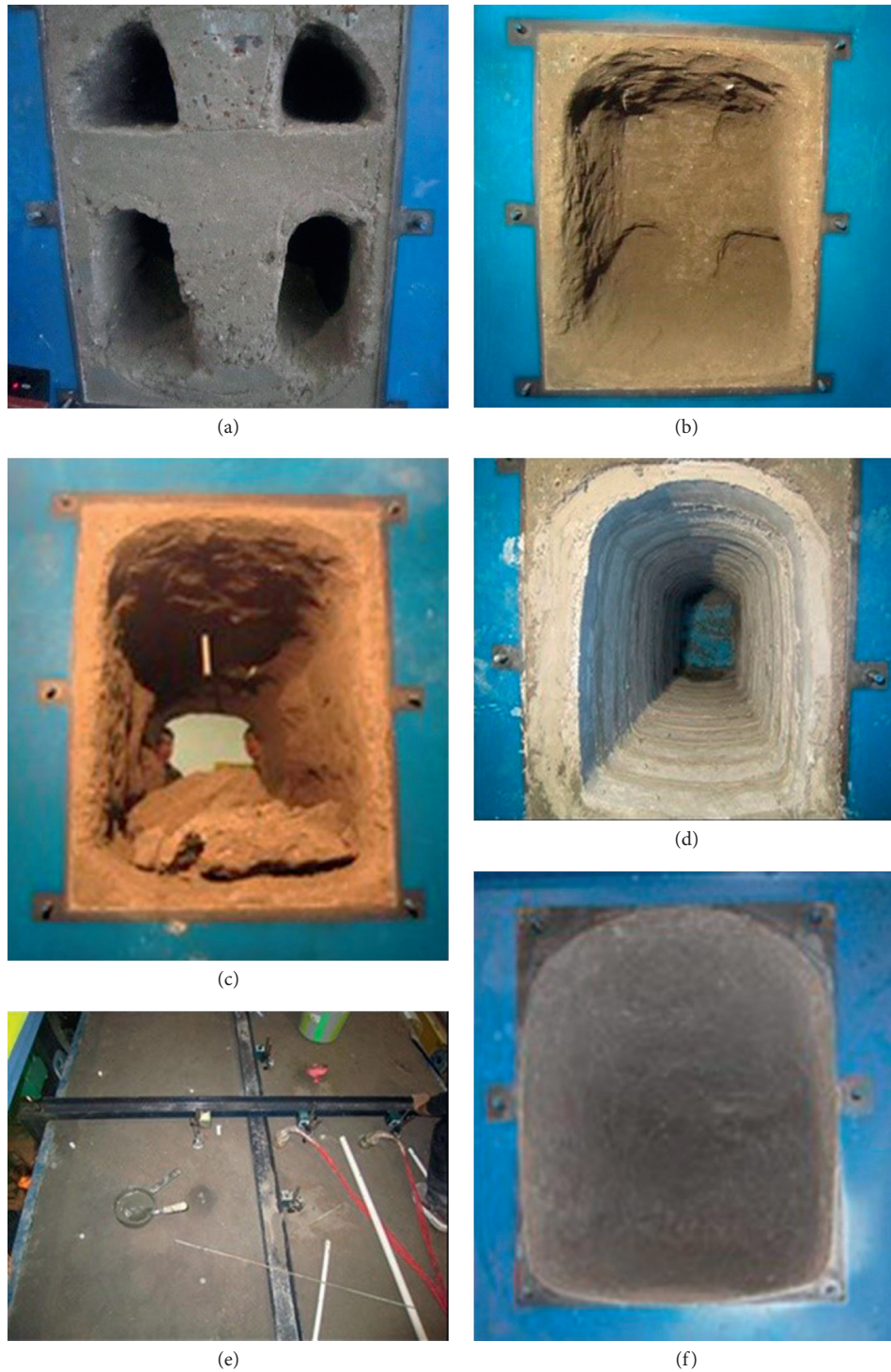
FIGURE 9: Model test excavation process: (a) step 1: four pilot headings when excavating the main tunnel for the first time; (b) step 4: excavating core soil and rock beam of the main tunnel for the second time; (c) step 6: excavating core soil and rock beam of the main tunnel for the third time; (d) step 9: secondary lining; (e) step 10: surface injecting; (f) step 14: fourth full-face excavation of the accessorial cross tunnel.
