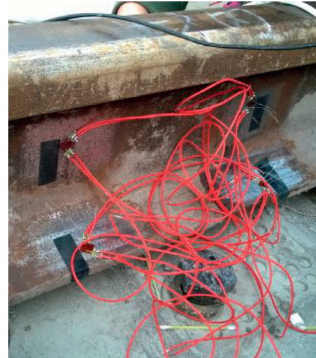
FIGURE 6: A scene from the field tests for the wheel-rail forces of a high-speed railway.
