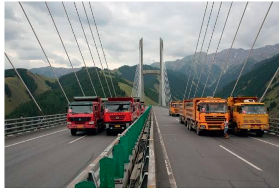
FIGURE 8: Live load test.
