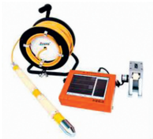
FIGURE 5: YL-LCT broken rock zone tester (Shanghai Y-Link Engineering and Technology Co., Ltd., China).
