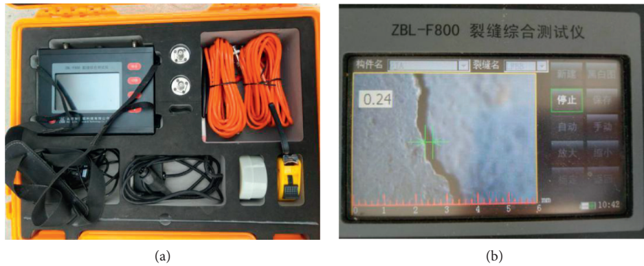
FIGURE 5: Comprehensive crack tester. (a) Tester. (b) Testing process.
