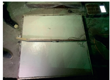
FIGURE 5: Composite panel production process. (a) Location of surface strain gauge. (b) Location of embedded strain gauge. (c) Mixing GRC. (d) Vibration rod vibration. (e) Roller brushing. (f) Smooth connection. (g) Rough connection. (h) Laying steel mesh connection. (i) Embedded strain gauge. (j) Surface strain gauge. (k) Fixed surface strain gauge.
