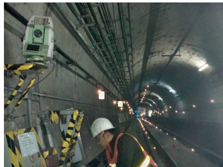
FIGURE 11: Automatic total station and reflection prism.
