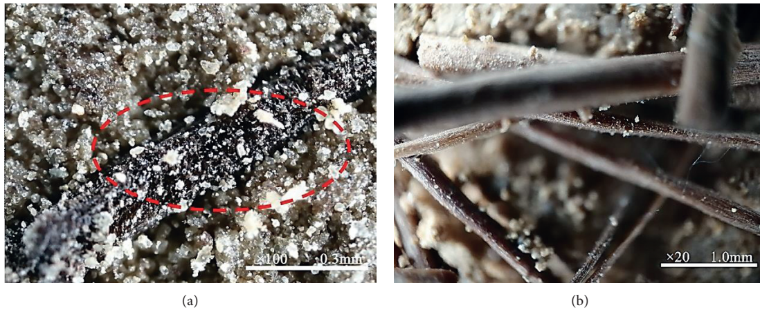
FIGURE 7: Distribution and surface characteristics of fibers in palm fiber-reinforced soil. (a) Single and (b) multiple fibers.
