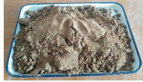
FIGURE 1: Saline soil used in test.
