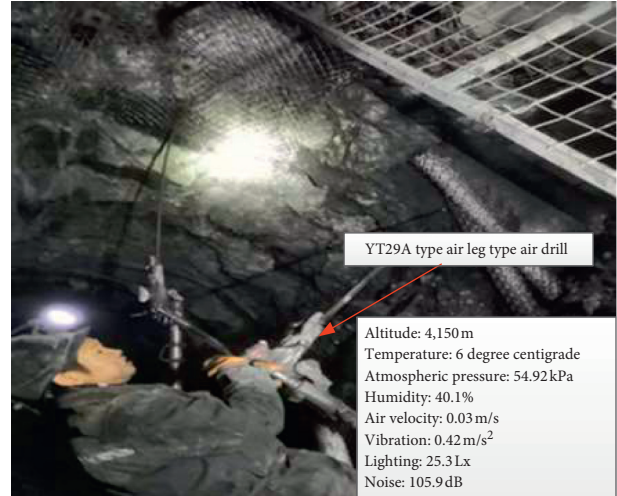
FIGURE 1: Air drill operation.
