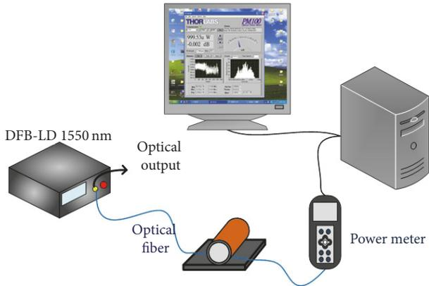
FIGURE 1: Schematic diagram of optical fiber polishing arrangement.
