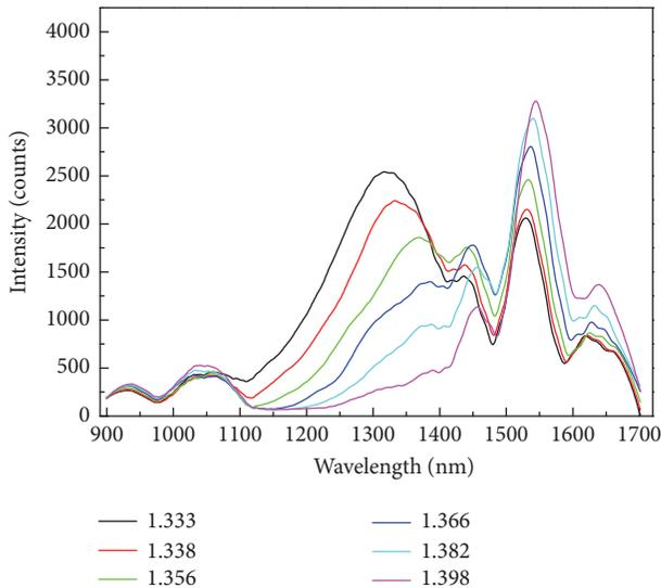
FIGURE 4: LMR spectra of the D-shaped fibers coated with  $\text{TiO}_2$  nanofilm for different liquid refractive indices.
