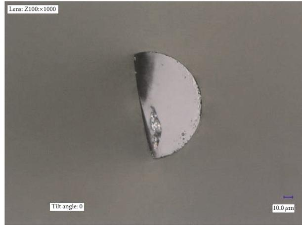
FIGURE 2: Microscopic image of the D-shaped fiber.
