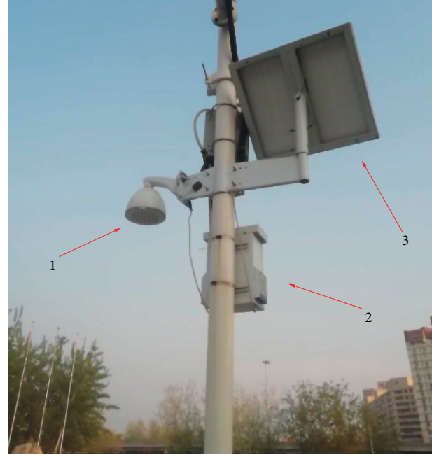
FIGURE 1: Air pollution monitor (1 is the device monitoring probe, 2 is the equipment power supply box, and 3 is the solar electronic board).
