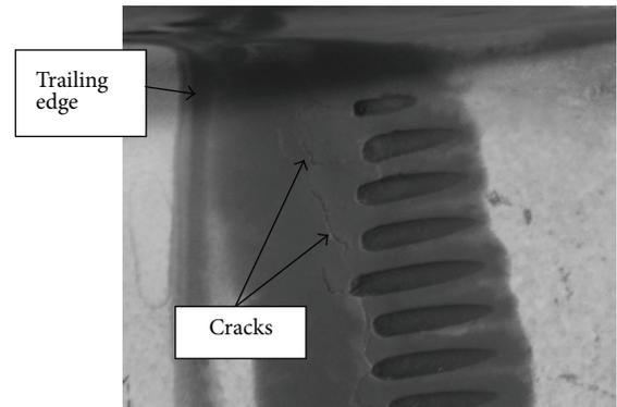
FIGURE 4: Cracks on the nozzle vane near the internal shroud close to the trailing edge.
