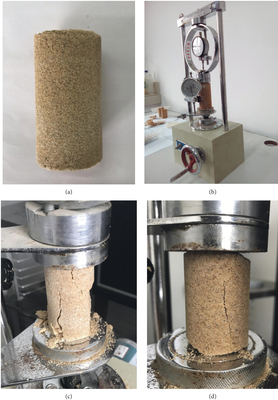
FIGURE 4: Photo of unconfined compression (UCC) strength tests: (a) MICP-treated sand specimen; (b) test setup; (c) specimen no. 3 at failure; (d) specimen no. 4 at failure.
