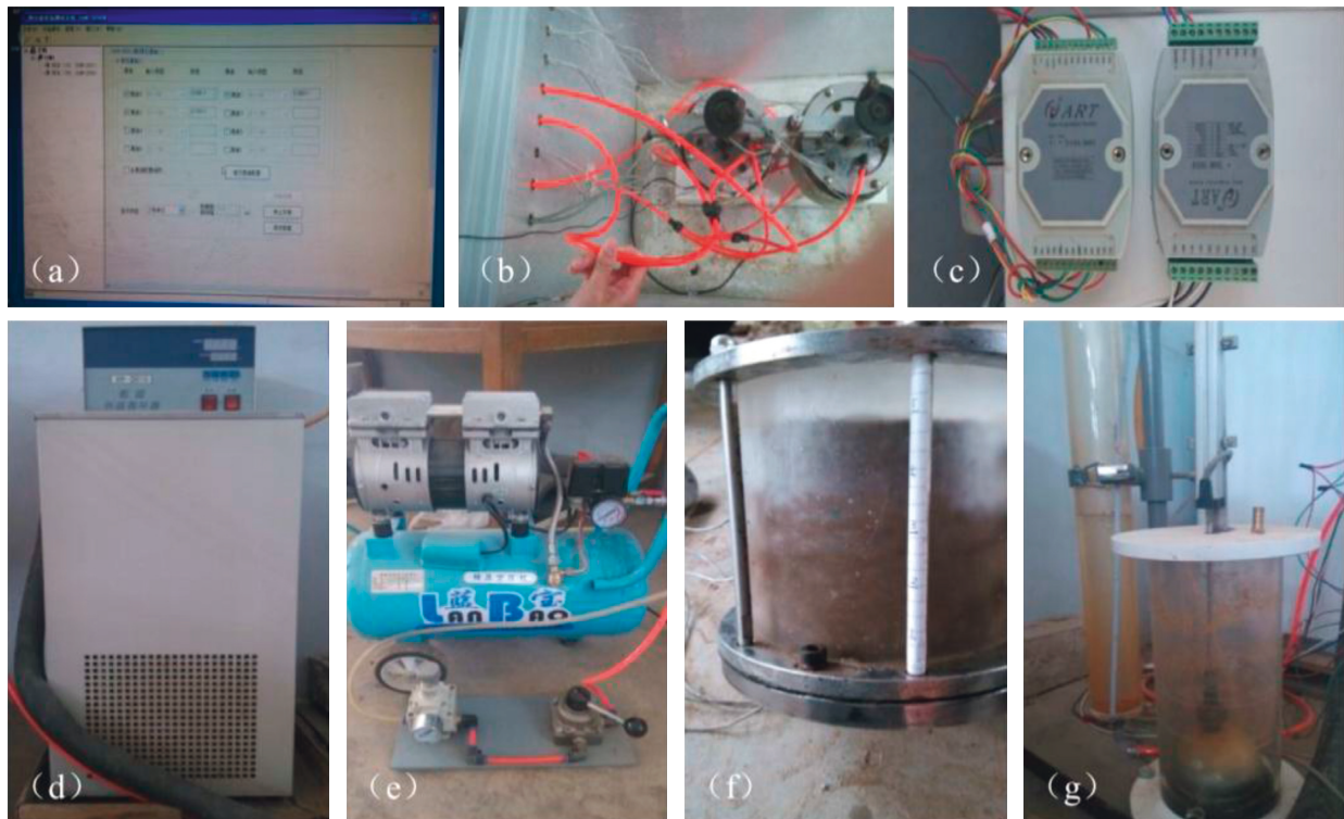
FIGURE 5: Improved frost heave experiment apparatus. (a) Altai measurement and control system. (b) Thermostat. (c) Data acquisition unit. (d) Cryostat. (e) Pneumatic balance apparatus. (f) Soil sample box. (g) Maddox water replenishing bottle.
