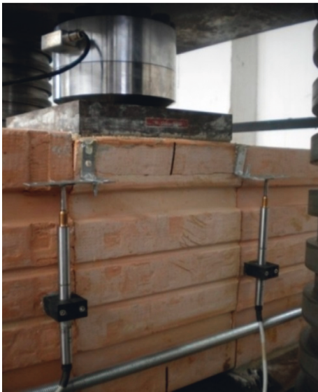
FIGURE 12: Second specimen failure under the maximum load.
