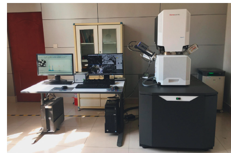
FIGURE 3: Apreo high-resolution SEM.
