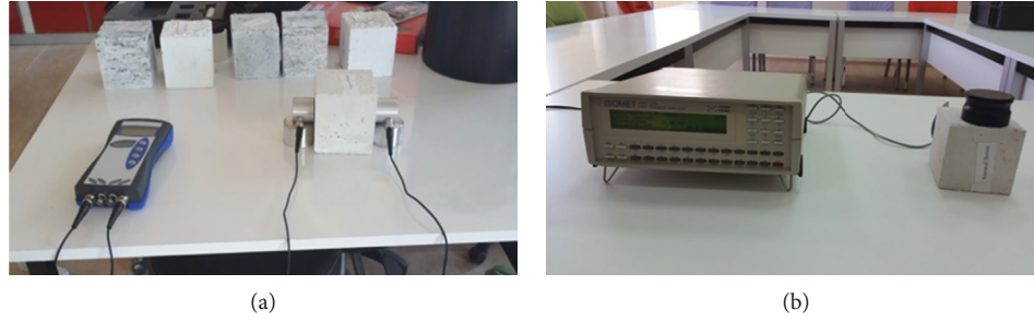
FIGURE 2: The measurement devices of ultrasonic pulse velocity and the thermal property.
