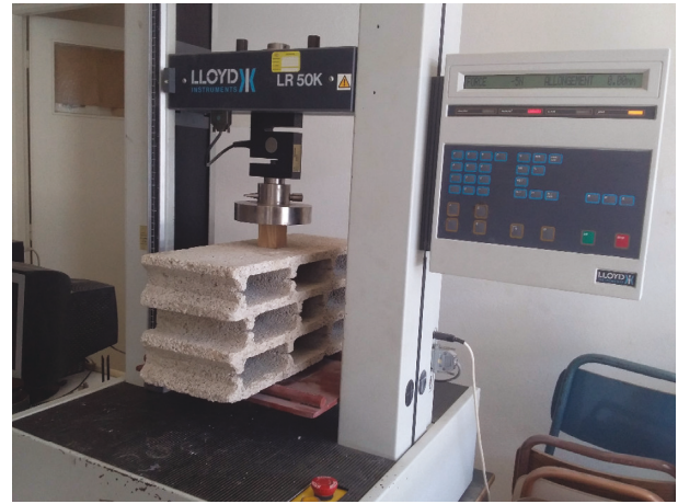
FIGURE 14: Punching-flexural test on the lightweight concrete block floor.
