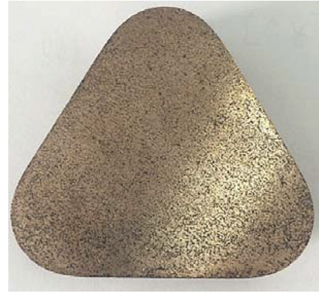
FIGURE 3: Surface of the brake pad after grinding.
