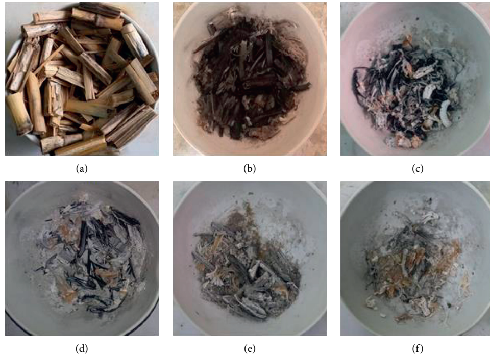
FIGURE 4: (a) Corn stalk. Color change at different temperatures: (b) CS400, (c) CS500, (d) CS600, (e) CS700, and (f) CS800.
