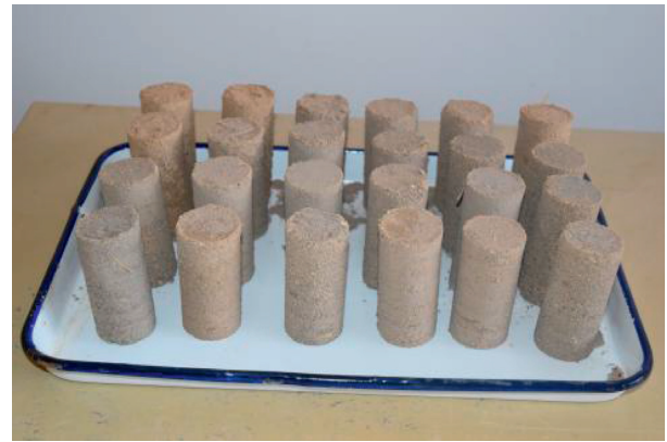
FIGURE 4: Specimens for unconfined compressive test.
