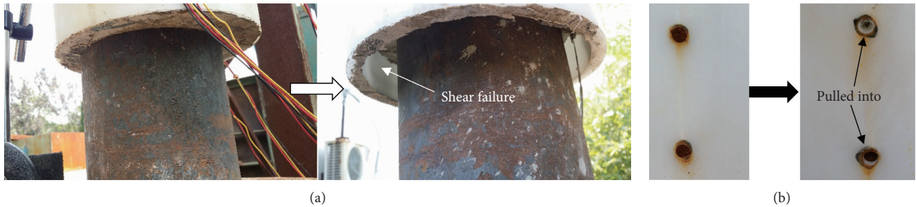
FIGURE 6: Failure modes of specimens. (a) Shear failure of FRP tube-concrete interface. (b) Shear connectors were pulled out.
