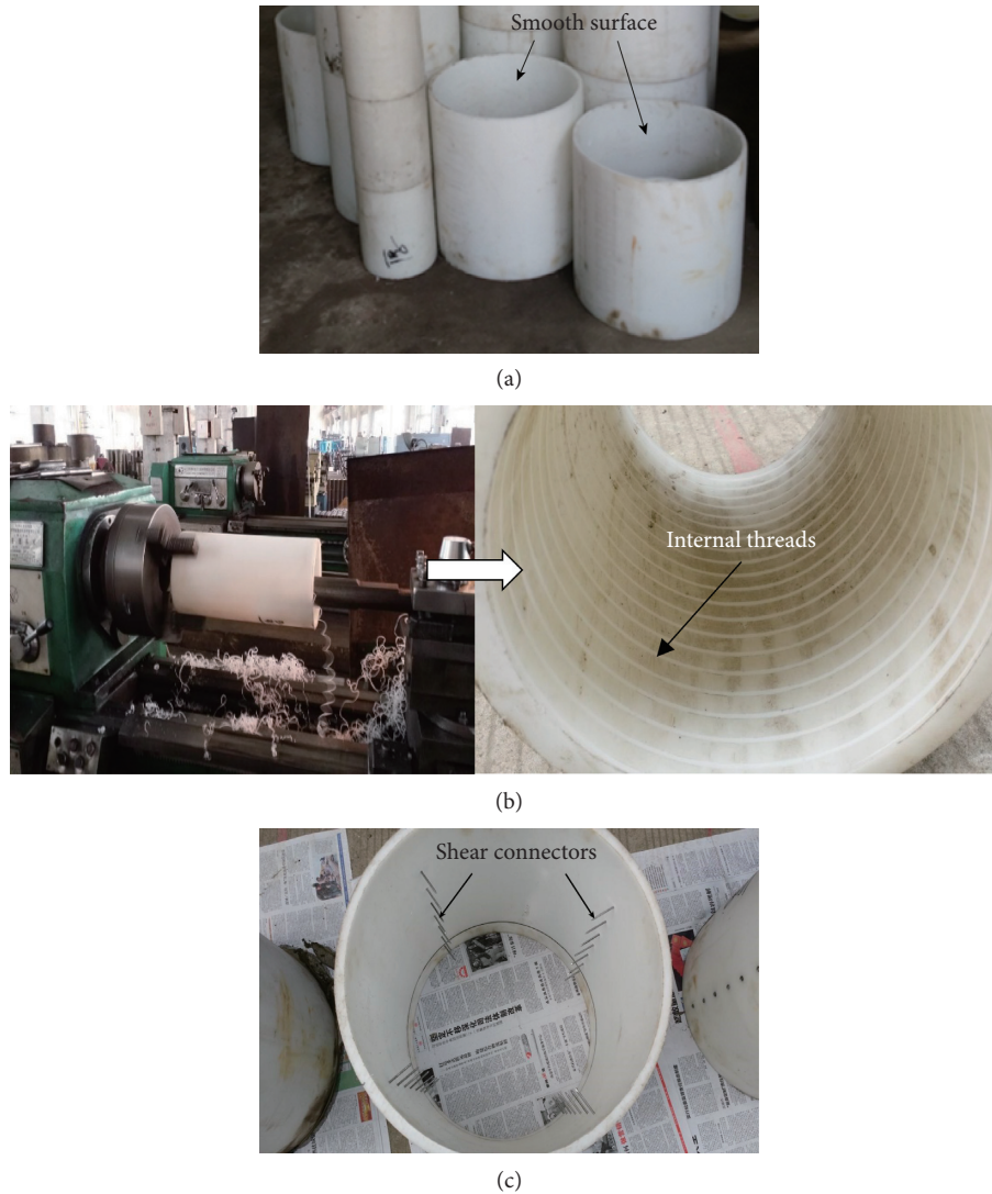
FIGURE 2: Different types of FRP tubes. (a) Normal FRP tubes. (b) FRP tube with internal threads. (c) FRP tube with shear connectors.
