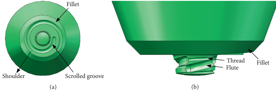
FIGURE 1: The tool used in welding experiments. (a) Vertical view; (b) front view.
