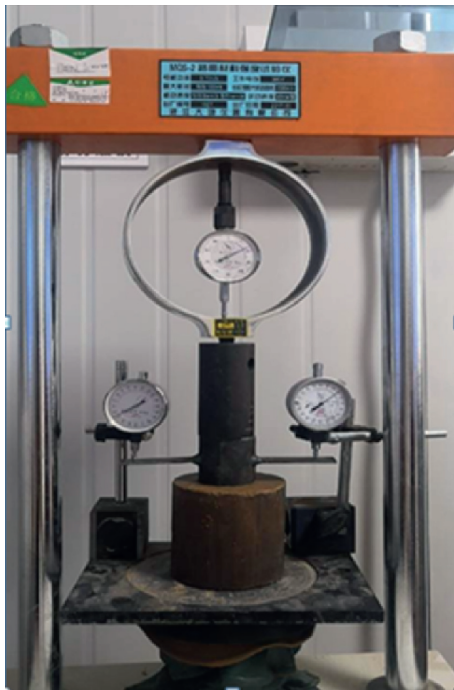
FIGURE 3: Photograph of resilient modulus test for CSL.
