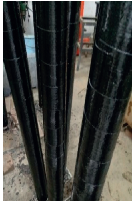
FIGURE 1: CFRP-CFST pile specimens.
