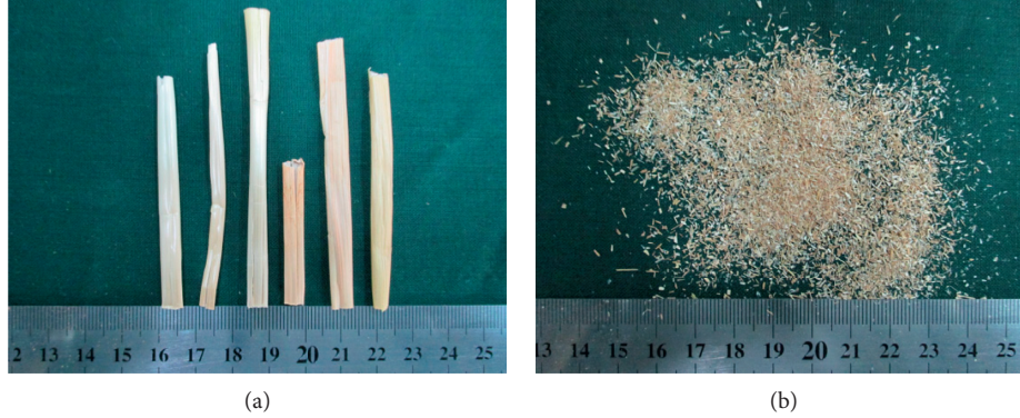
FIGURE 1: Appearance of wheat straw and wheat straw fiber. (a)Wheat straw. (b) Wheat straw fiber (particle size 0.3 mm).
