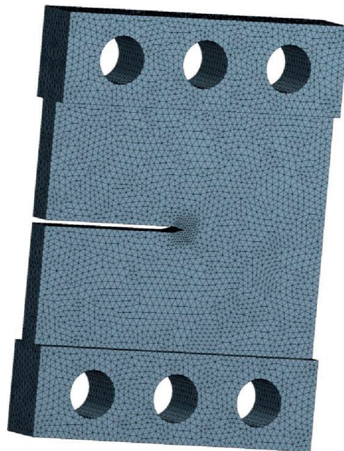
FIGURE 3: 3D ANSYS model for CTS specimen (no. of nodes = 201317 and no. of elements = 132886).
