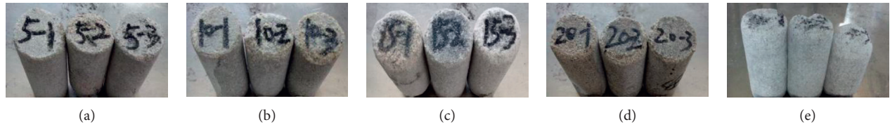
FIGURE 4: Apparent properties of the feldspar sandstones (group B) after a salt-rock dry-wet cycle. (a) 5 T. (b) 10 T. (c) 15 T. (d) 20 T. (e) 25 T.
