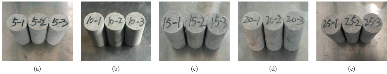
FIGURE 3: Apparent properties of the feldspar sandstones (group A) after a water-rock dry-wet cycle. (a) 5 T. (b) 10 T. (c) 15 T. (d) 20 T. (e) 25 T.
