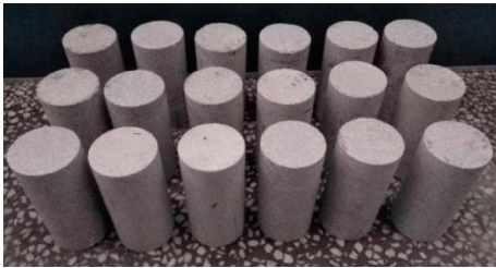
FIGURE 2: Standard feldspar sandstone samples.
