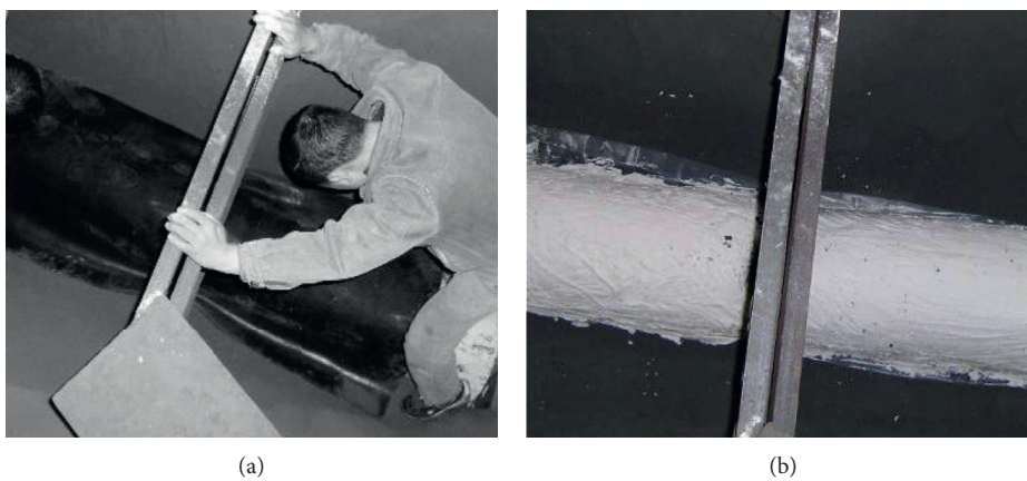
FIGURE 4: Test similar material. (a) The reducing dislocation layer. (b) Flashing and primary support.
