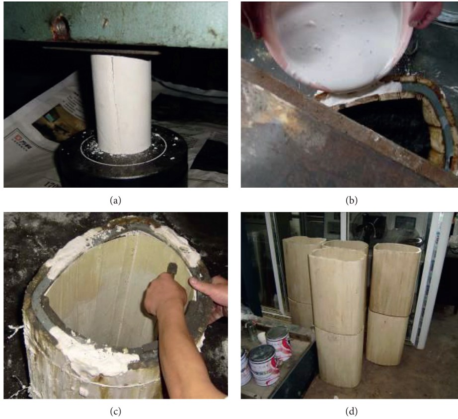
FIGURE 3: Secondary lining model. (a) Lining similar material mechanics test. (b) Lining model pouring. (c) Mold stripping. (d) Airing and lacquering.
