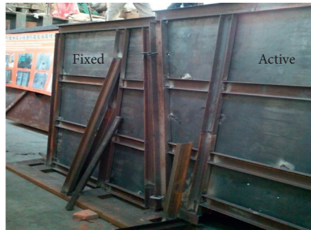
FIGURE 1: Stick-slip dislocation test box.
