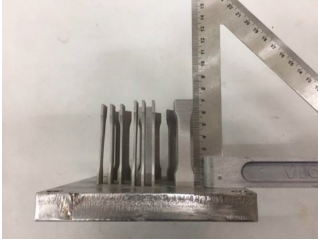
FIGURE 4: Physical image of the tensile specimen after heat treatment.
