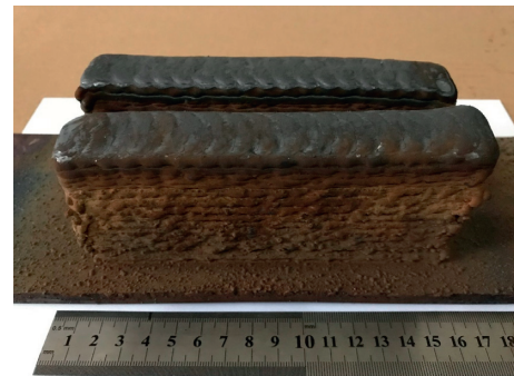
FIGURE 1: Schematic of a 2.25Cr1Mo0.25V heat-resistant steel sample produced by WAAM.
