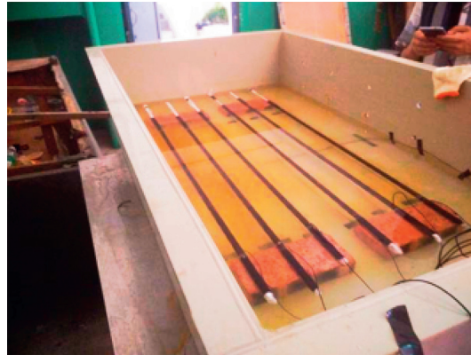
FIGURE 5: Corrosion diagram of steel strands.
