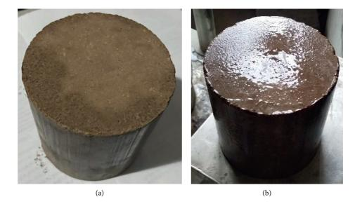
FIGURE 5: Photographs of specimens before and after the eroding test. (a) Specimen not tested in the eroding test. (b) Specimen after an eroding test for 30 min.
