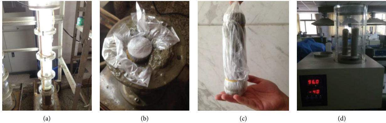
FIGURE 4: Process of pretreatment by the freeze-drying method. (a) Settling column. (b) Underflow sample. (c) Sample holder. (d) Vacuum freeze-drying machine.
