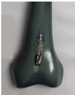
FIGURE 2: Eccentric reaming of the anterior cortex using a 10 mm diameter reamer created the anterior cortical perforation of the distal femur for the POS-P nail group. The reamer was advanced further than shown, until the full size of the perforation was made.
