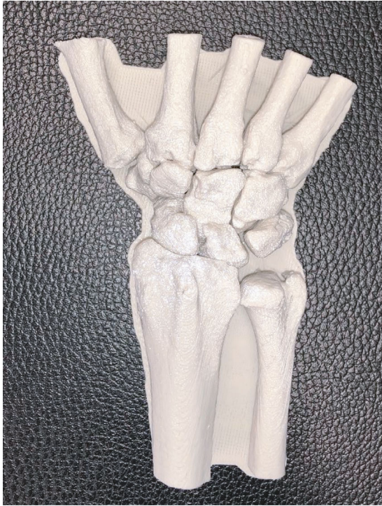
FIGURE 1: 1 : 1 model based on 3D-Computertomography (CT) data of the carpal bones printed on an FDM-printer. This model allows analysis of intracarpal relationships und surgical training.
