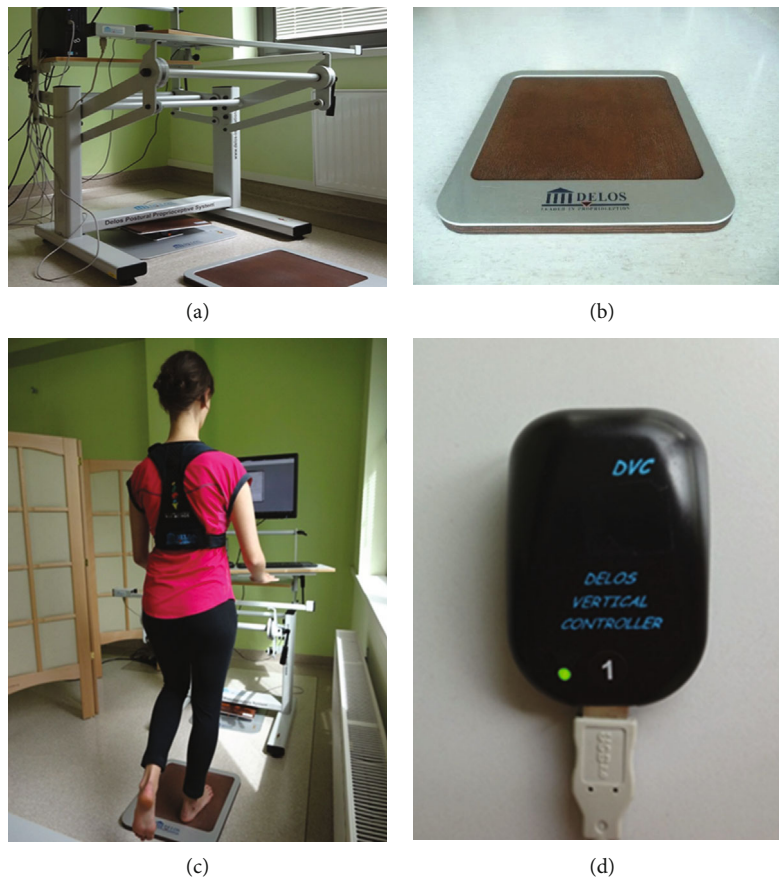
FIGURE 2: Delos postural proprioceptive system: (a) the postural proprioceptive station, (b) Delos Equilibrium Board, (c) position during Static Riva Test, and (d) Delos Vertical Controller.
