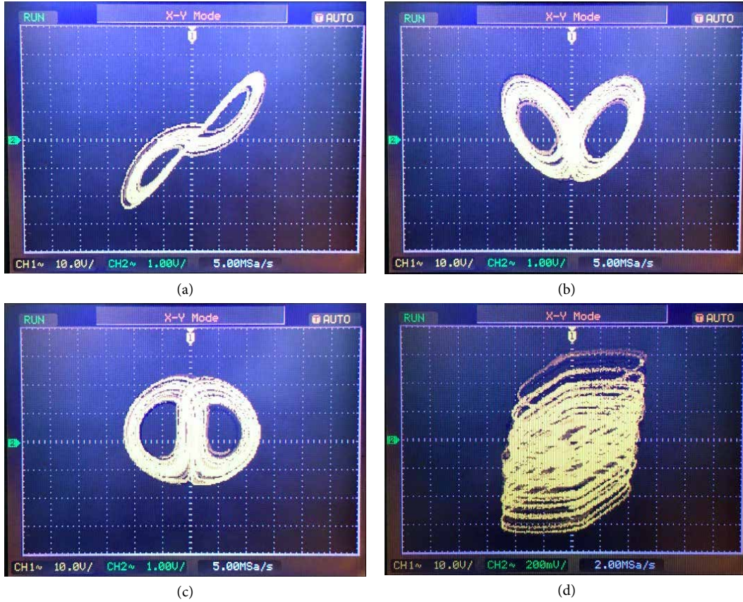
FIGURE 13: Chaotic attractors observed from an analog oscilloscope. (a) x - y plane; (b) x - z plane; (c) y - z plane; (d) x - w plane.
