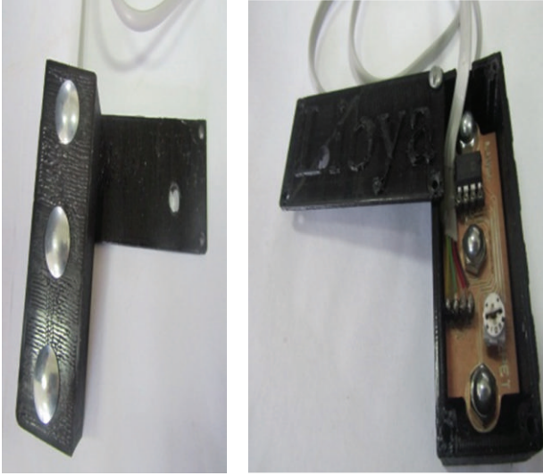
FIGURE 7: The double sides of sensor circuit designed by EPET.
