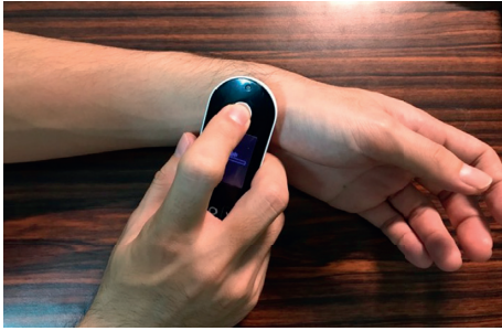
FIGURE 2: Freescan measurement: the right hand is used to hold the Freescan instrument to measure pulse site on the left hand.
